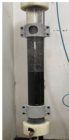
Figure 2. Inverse Fluidized Bed of the AHR.
