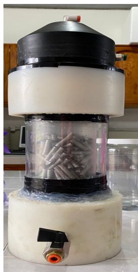
Figure 1. Fixed Bed of the AHR.
