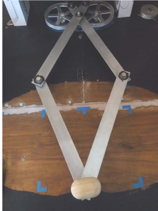
Fig 1: Main structure of the parallel planar robot
