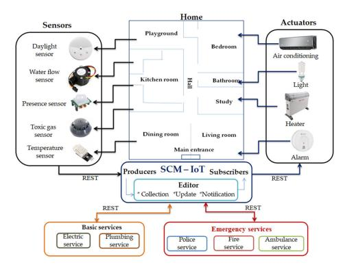
Figure 1. SCM-IoT deployment scenario.
