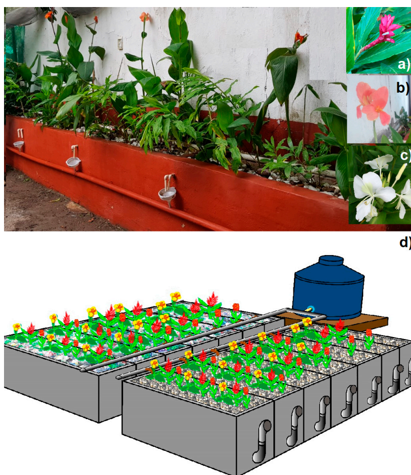
Figure 6. Constructed wetland systems. (a) Alpinia purpurata , (b) Canna hybrids , (c) Hedychium coronarium , (d) Scheme of CWs in study.
